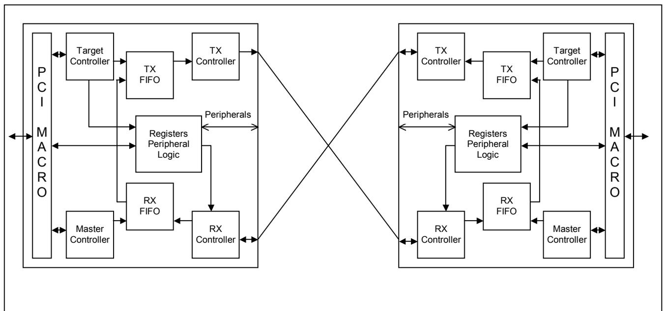
Figure 1. System Level Block Diagram
